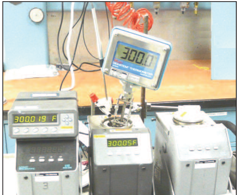
Wahl DST600 Series thermometer system being tested in the calibration lab of a major food processor, against two certified references.
